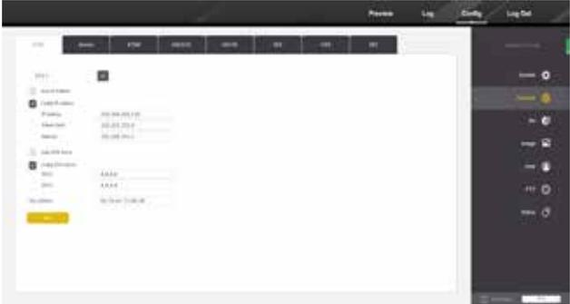
**[EHP]** : Set the IP address and its DNS Server of the device. Note that the IP address is consistent with the gateway, and the Mac address cannot be modified.
