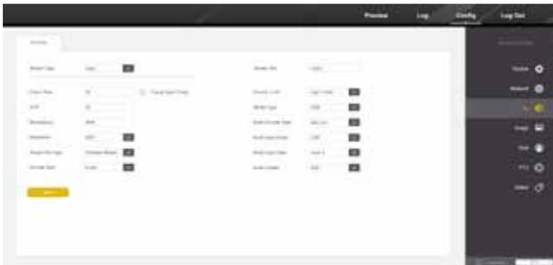
**【Stream Type】** : You can choose the main and second streams. and The user configures the parameters of the corresponding stream according to the needs (the web page generally uses the main stream and cannot be changed)
