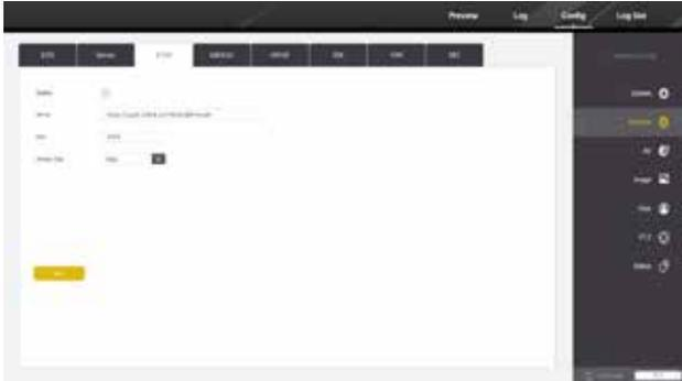
**【Server】** : RTMP server address, generally used for webcasting, obtain the RTMP streaming server address (usually `rtmp://IP address: port /platform live segment/platform live code`) on its live broadcast platform, and copy it Go to "Server Address", turn on the streaming switch, and click Save to preview the screen on the platform.
