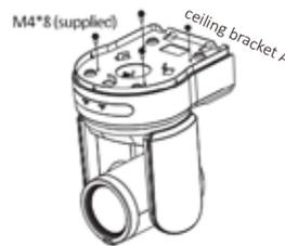
**3.** Fasten the safety wires to the ceiling brackets A and B respectively. Make sure that the triangle marks of ceiling bracket A and bracket B are aligned as shown in the figure, and then rotate the camera clockwise so that ceiling bracket A and bracket B are fully locked.
