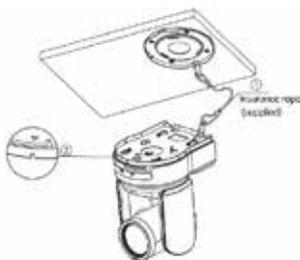
**4.** Fix ceiling brackets A and B using the three screws provided (M3 X 8).
